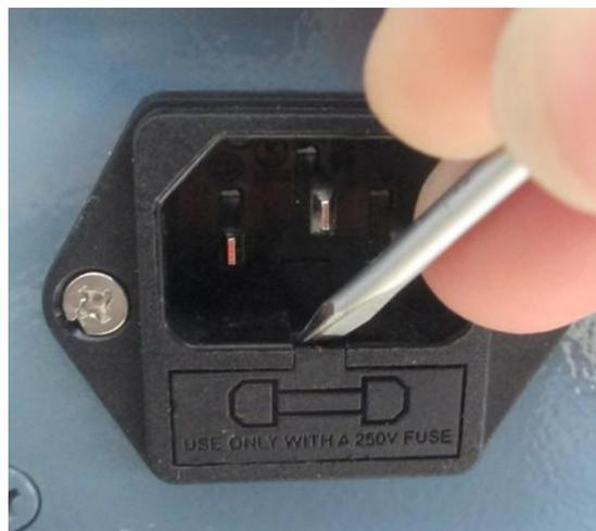
Step 3: Pull out the holder, the fuse is inside it.
