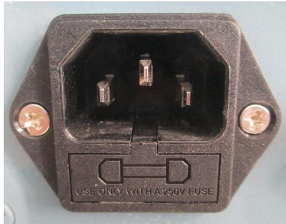
Step2: Prepare a flat screwdriver, open the black cover as picture below.
